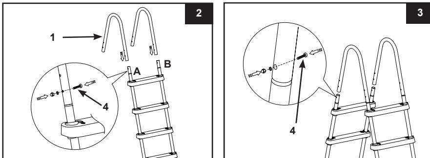
**3. INSTALLATION OF THE REMAINING LADDER SIDE** (refer to figure 3):**4. TOP BRACE INSTALLATION – ONE SIDE AT A TIME** (refer to figure 4):
